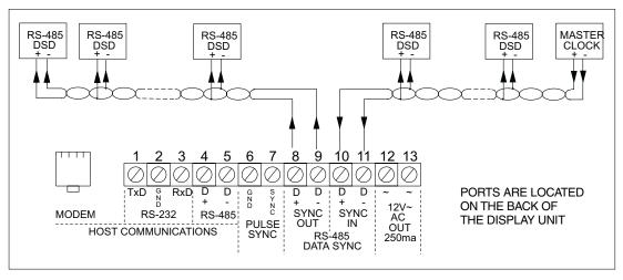
Figure C-8 Synchronizing RS-485 Time Synchronization Devices Without a Buffer
